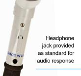
The receiver is handheld and light with the meter fitted at the top of the 48 inch long instrument
